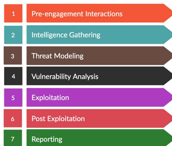
Gambar 1. Penetration Testing Life Cycle berbasis PTES
